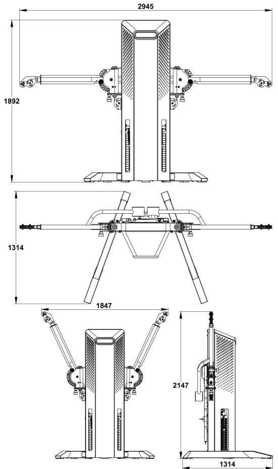
Assembled Dimension: 1314mm x2945mm x2147mm
